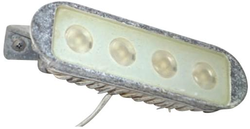
*A powder coated aluminum floodlight with housing degradation*
